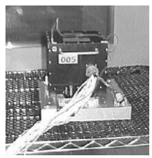
An Inertial Reference Unit (IRU) in a temperature test chamber at Honeywell.
